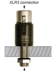
1/8" pipe nipple or "lamp pipe" bushing. Can be any length; one inch is normally supplied for table surfaces 3/4" or less in thickness. Drill 7/16" hole.
